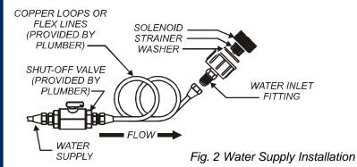
In some areas, local codes require a backflow preventer (check valve) to be installed on the inlet water line. If a backflow preventer is used, you must install a *water hammer arrester* in the incoming line, between the backflow preventer and the brewer inlet, as far away from the brewer as space will allow. This will relieve the excessive back pressures that can cause faucet leaks and solenoid malfunctions.
